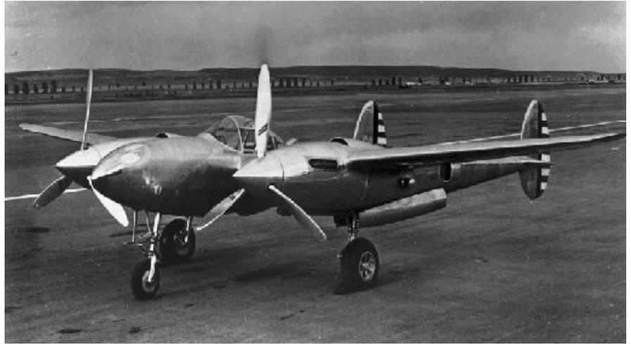
The tail dragged on the runway. Damage was minor and the problem was quickly solved. Designed by an engineering team led by Hall L. Hibbard, which included the legendary Clarence L. "Kelly" Johnson, the XP-38 was a single-place, twin-engine fighter designed for very high speed and long range. It was an unusual configuration with the cockpit and armament in a center nacelle, with two longitudinal booms containing the engines and propellers, turbochargers, radiators and coolers.
