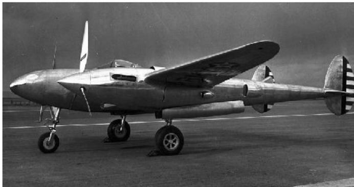
variable-pitch propellers inward to counteract the torque effect of the engines and propellers. The XP-38 had a maximum speed of 413 miles per hour at 20,000 feet and a service ceiling of 38,000 feet. The XP-38 was unarmed, but almost all production Lightnings carried a 20 mm auto cannon and four Browning .50-caliber machine guns grouped together in the nose. They could also carry bombs or rockets and jettisonable external fuel tanks.
